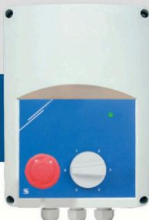
The SER-1 series of transformer fan speed controllers regulate the rotational speed of single-phase voltage controllable motors by varying the output voltage. They are equipped with an auto-transformer and control the speed manually in five steps. The technology used provides a regulated output voltage with a perfect sinusoidal shape. The controllers feature an emergency button for smoke extraction.
